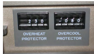
Chamber safety includes an overheat/overcool to protect the chamber and test load, and an emergency stop switch.
